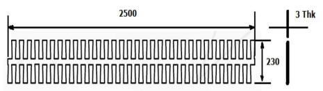
To ensure that a vault is safe, a vault must be inaccessible from every direction and that includes walls floors and roof slabs. To make the vault inaccessible Gunnebo offers Gunnebo Tang Bars, which inhibits any unauthorized admittance into the vault through the vault.
